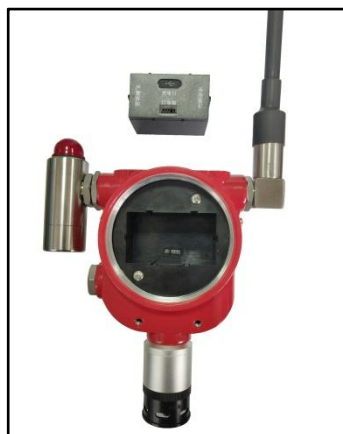
b. Replace the main power supply
