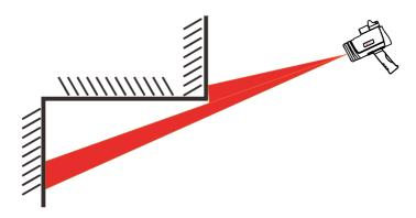
[3] When detecting a corner against a high reflectance background, two reflection points of spotter laser can be observed. At this time, false alarms may be caused, and other angles should be changed to test again to determine whether it is a leak alarm.
