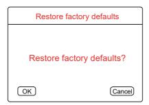
On the main menu interface, move the cursor with the  $\langle\!\langle \langle \rangle \rangle\!\rangle$  keys to select the factory reset icon, and press M key to enter the factory reset. Press M key to restore the factory and return to the main menu.
