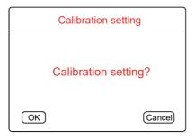
On the main menu interface, move the cursor with the  $\langle\!\langle \, \langle \, \rangle \, \rangle\!\rangle$  keys to select the calibration setting icon, and press the M key to enter the calibration setting.
