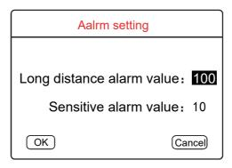
After selecting the alarm setting, press the M key to enter the alarm setting; "Long distance alarm value" is the alarm minimum value in remote mode, and "Sensitive alarm value" is the fluctuation value alarm in high sensitivity mode. After selecting the alarm value, press the M key to select the value, and adjust the  $\langle\langle\langle \rangle\rangle\rangle\rangle\rangle$  keys to change the alarm threshold.
