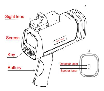
ARD3000 Remote Methane Leak Detector is suitable for remote measurement of methane gas leakage. It emits two light beams, one is a visible spotter laser (green), used to point to suspected leaks; the other is an invisible detector laser, used to measure the concentration of methane at the leak, and the concentration unit is ppm.m.
